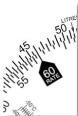
First we set up for the fuel flow: 46 litres per hour means we need to set 46 over 60 on the flight computer. We want to know the number of litres burnt in 111 minutes so the next step is to find 111 minutes on the inner scale and read the litres off the outer scale - **85** litres.
