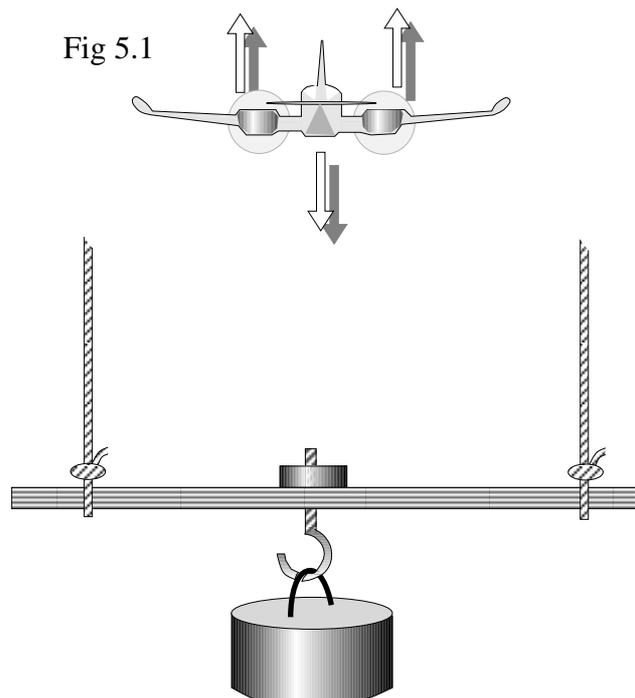
If the weight is increased the bending loads imposed on the plank will increase until the plank breaks under the increased load [Fig 5.2 top].
