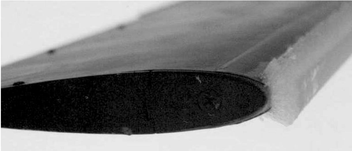
Rime ice which has formed on the leading edge of a helicopter rotor blade. Note that the ice builds up on the leading edge of the blade leaving the top and bottom surfaces virtually ice free. The ice build-up acts as a spoiler, disrupting the airflow over the aerofoil surface and drastically affecting the lift produced.
