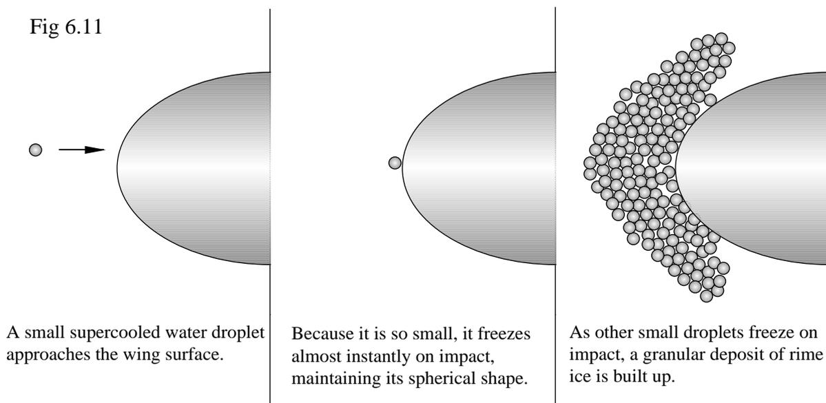
The relative size of the droplets in the figure above has been greatly exaggerated for clarity. The deposit of rime ice grows on the leading edges in a mushroom shape causing disruption to the oncoming airflow. This reduces lift and increases drag, requiring a greater angle of attack to compensate. The aircraft performance can be seriously impaired. Rime ice also forms over pitot tubes, depriving the pilot of airspeed indication.
