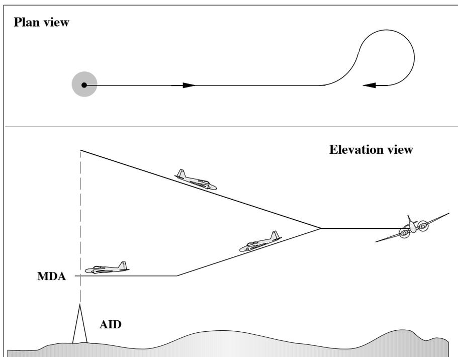
A typical non precision approach is shown in the figure above. From overhead the aid the pilot tracks outbound on the specified track descending to not below a specified level. He then carries out a procedure turn to place the aircraft inbound to the aid on the reciprocal of the out bound track. He continues the descent to the published MDA.
