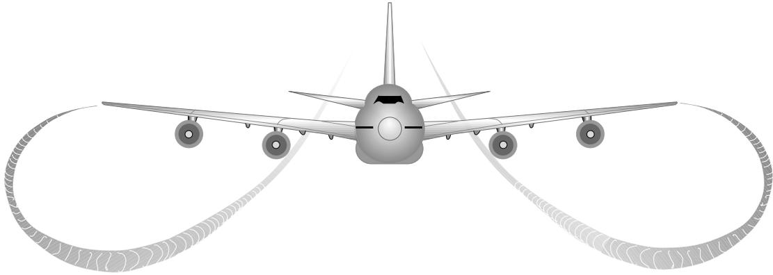
Vortices sink down at a rate of about 500 feet per minute until they reach a level about 700 to 1000 feet below the flight path
