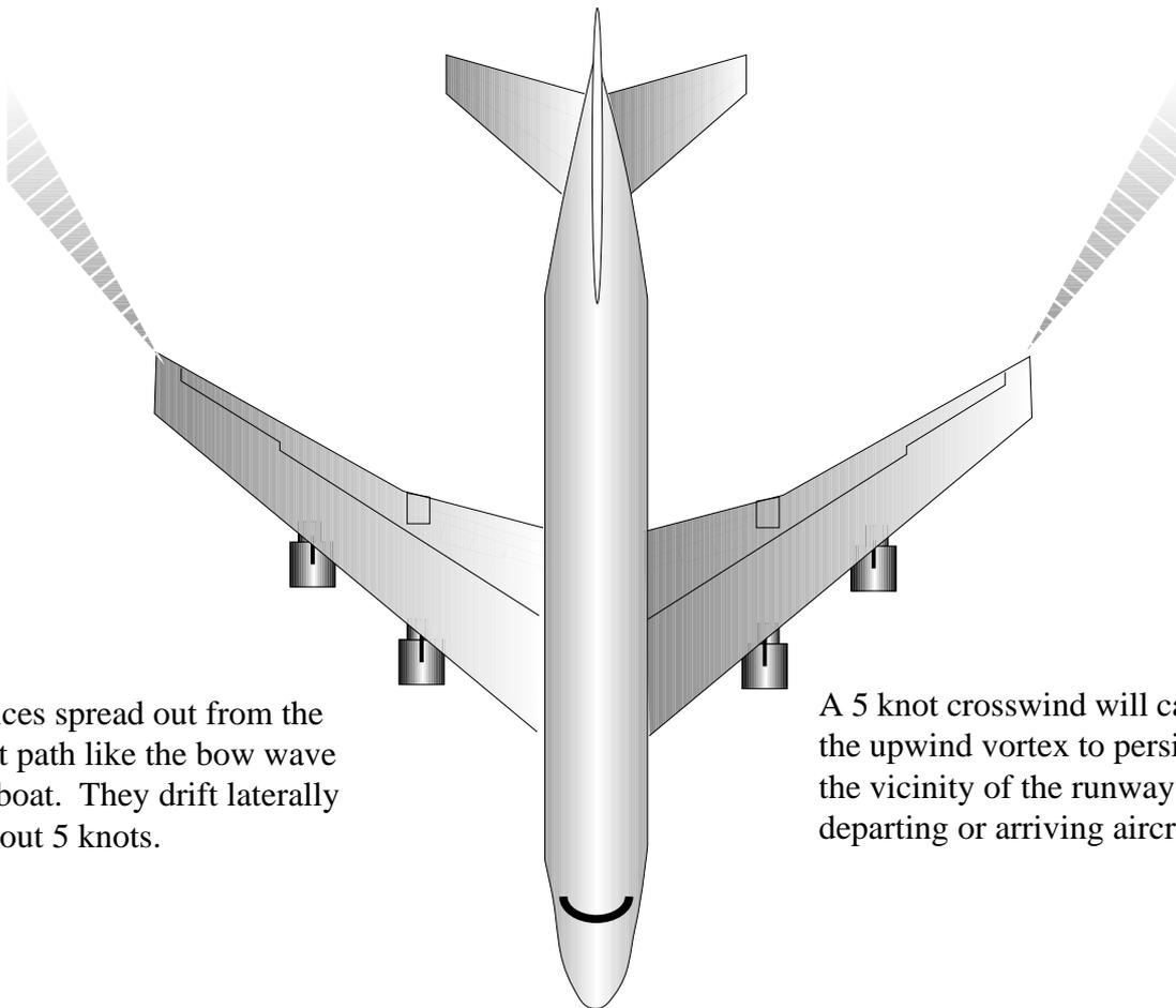
Vortices spread out from the flight path like the bow wave of a boat. They drift laterally at about 5 knots.
